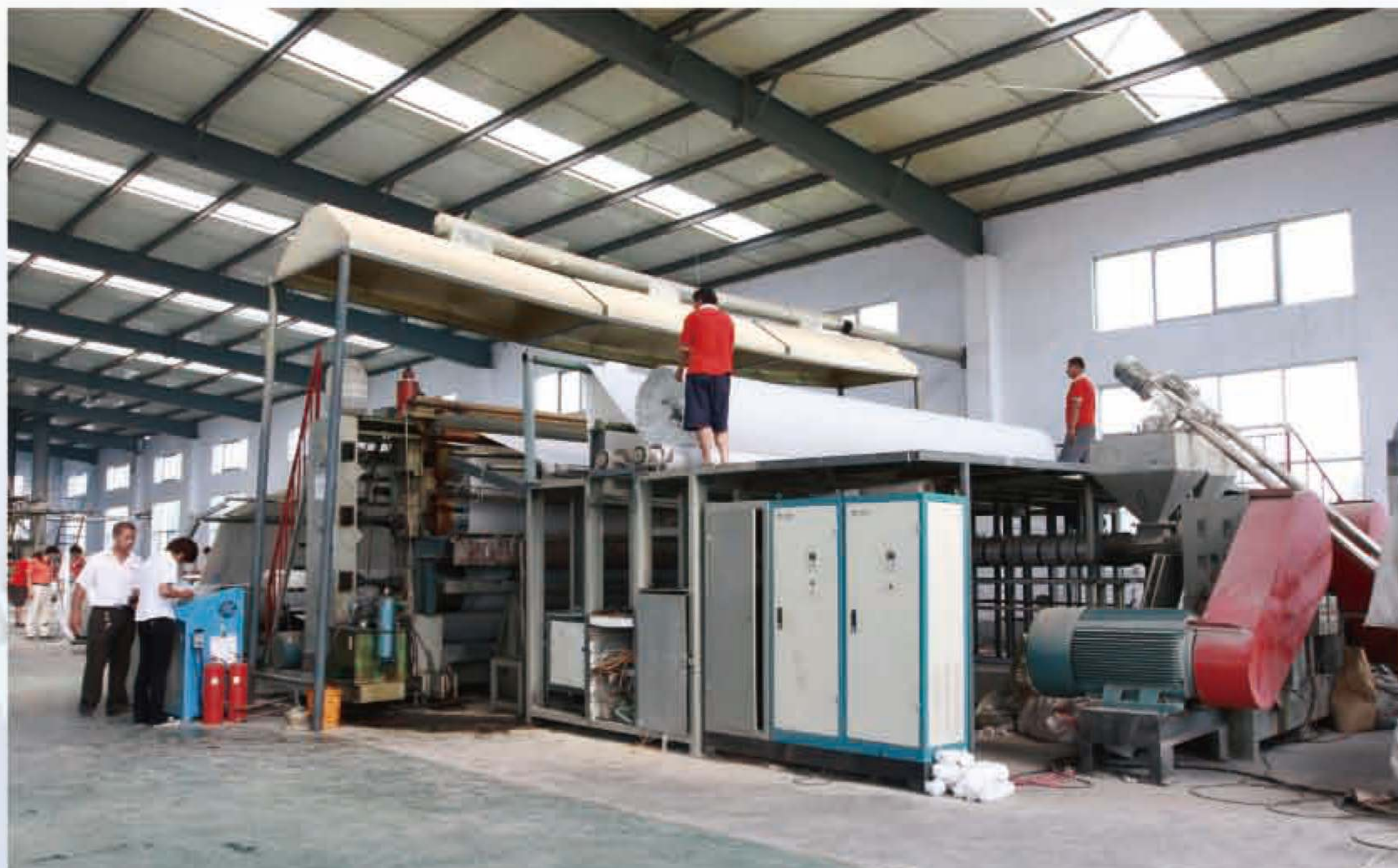
淋膜生产线 Drip washing geomembrane production line
