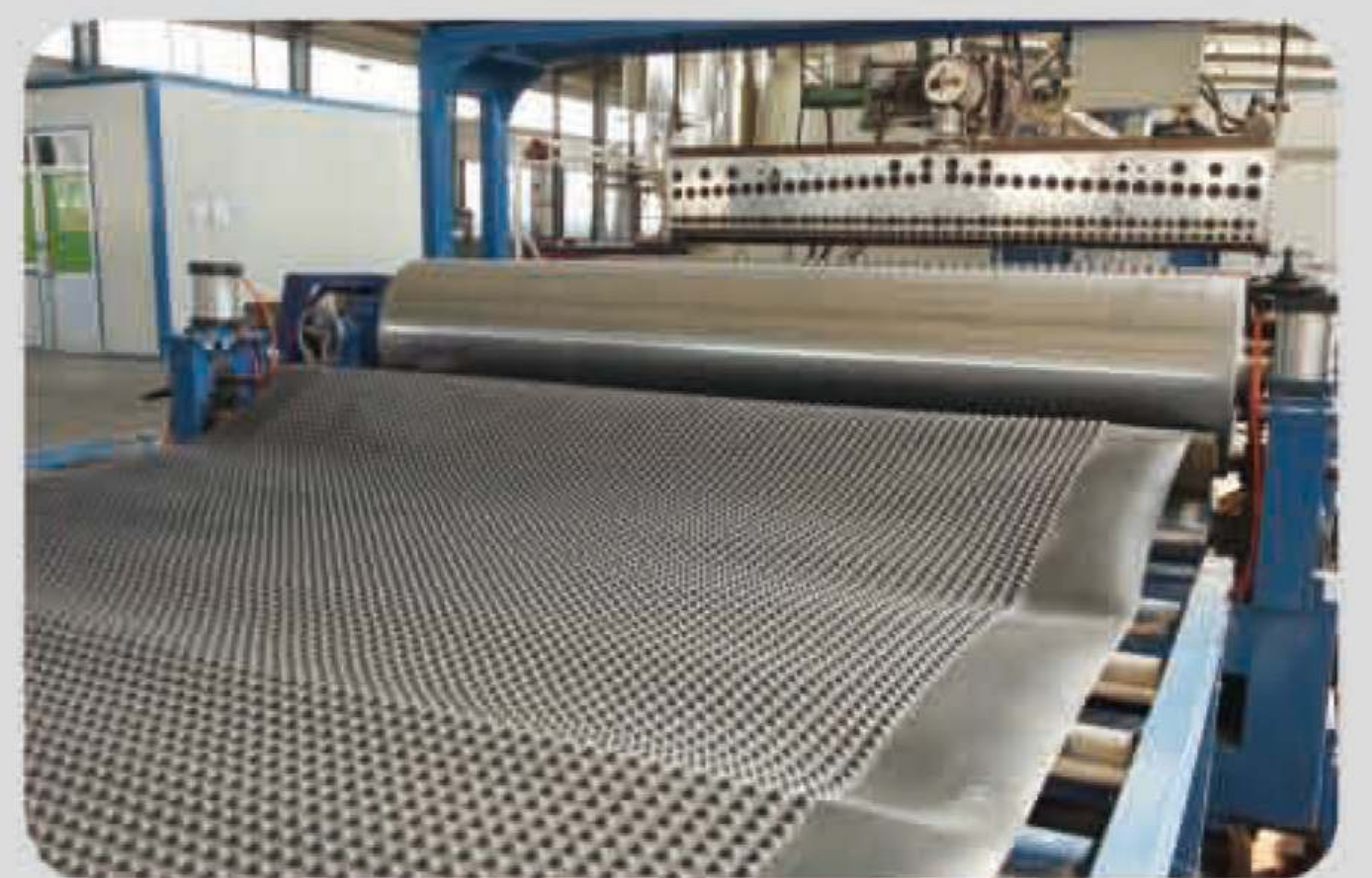
组合式防排储水隔离板生产线 Drainage board production line
