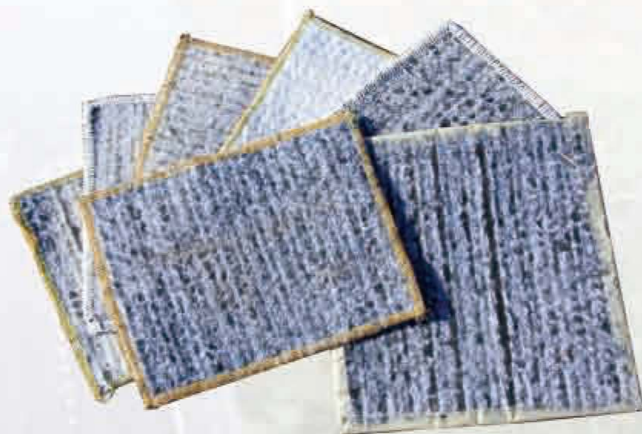
膨润土防水毯 (GCL) Geosynthetic Clay Liner
