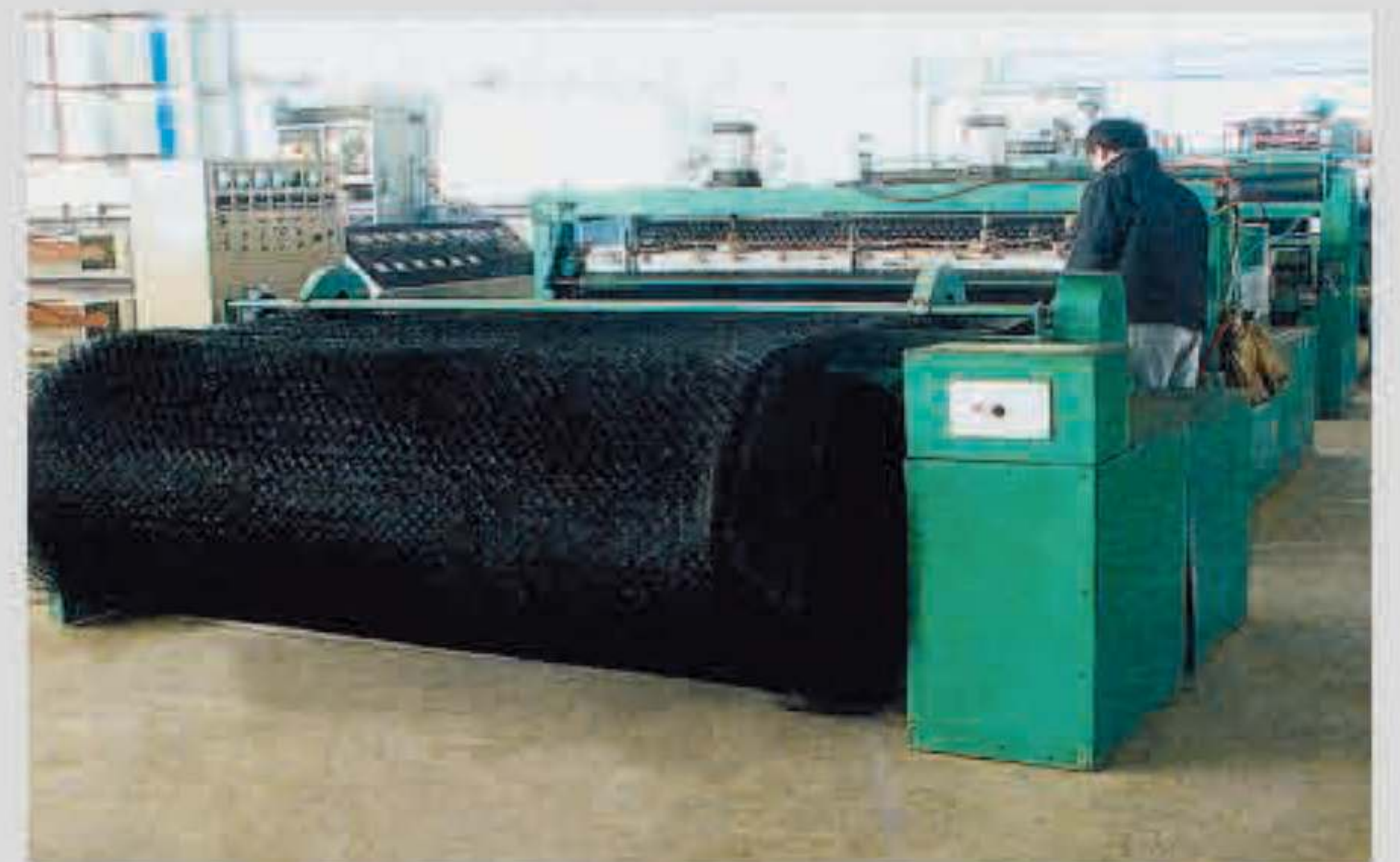
土工三维固土网垫生产线 Production line of Tri-dimension geomat for soil-fixing
