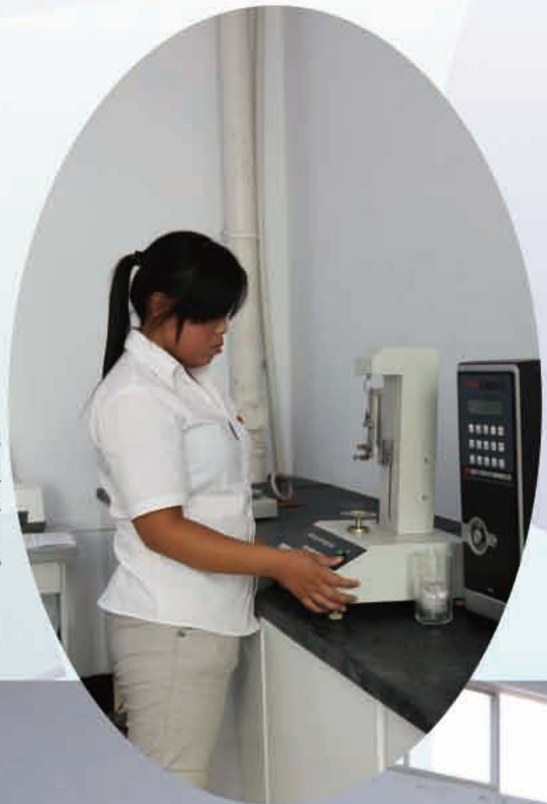
纤维强力机 Fiber strength testing machine
