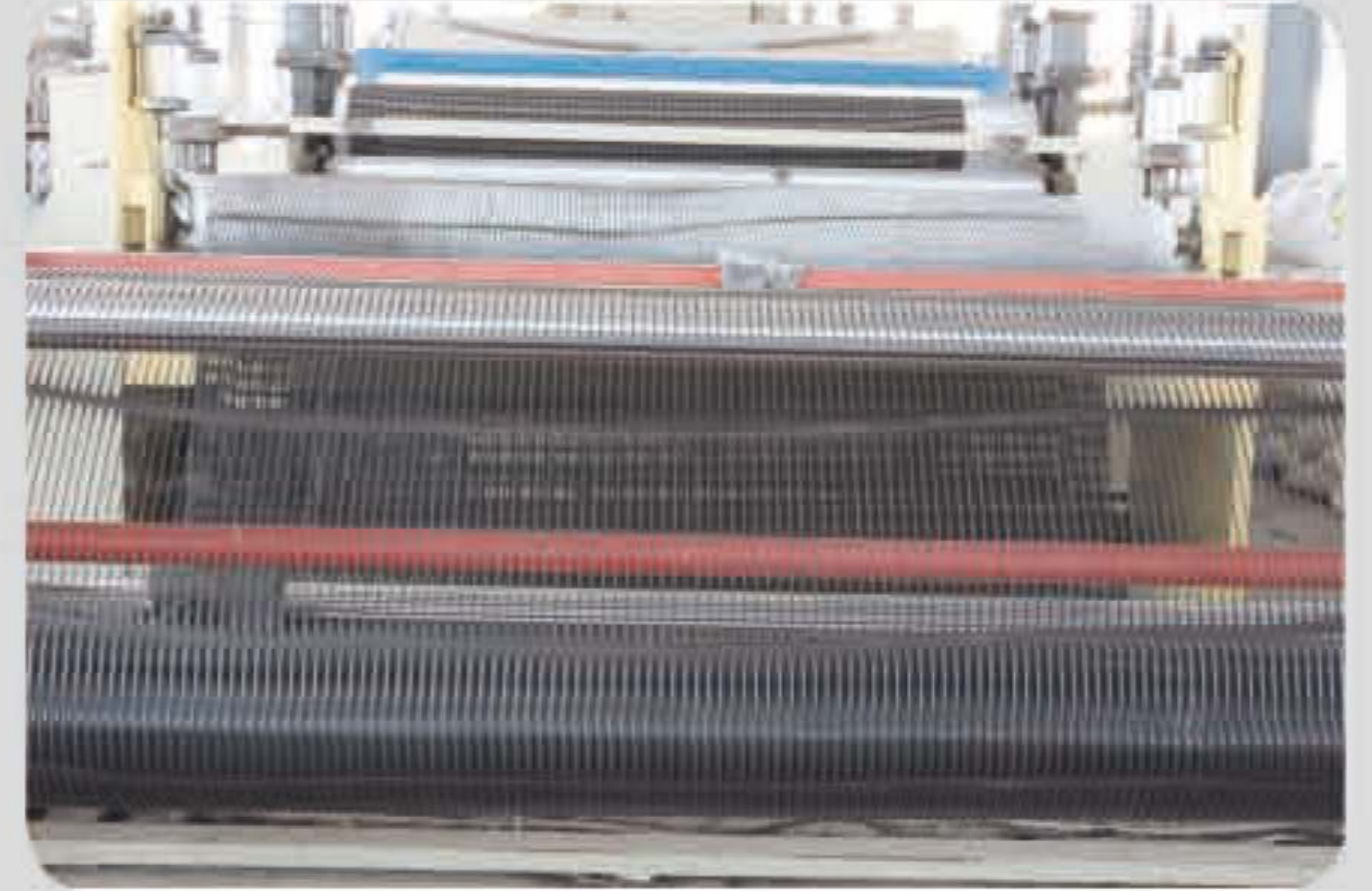
高强加筋单向格栅（宽2.5米）生产线 Single direction geogrid production line, 2.5 meters in width
