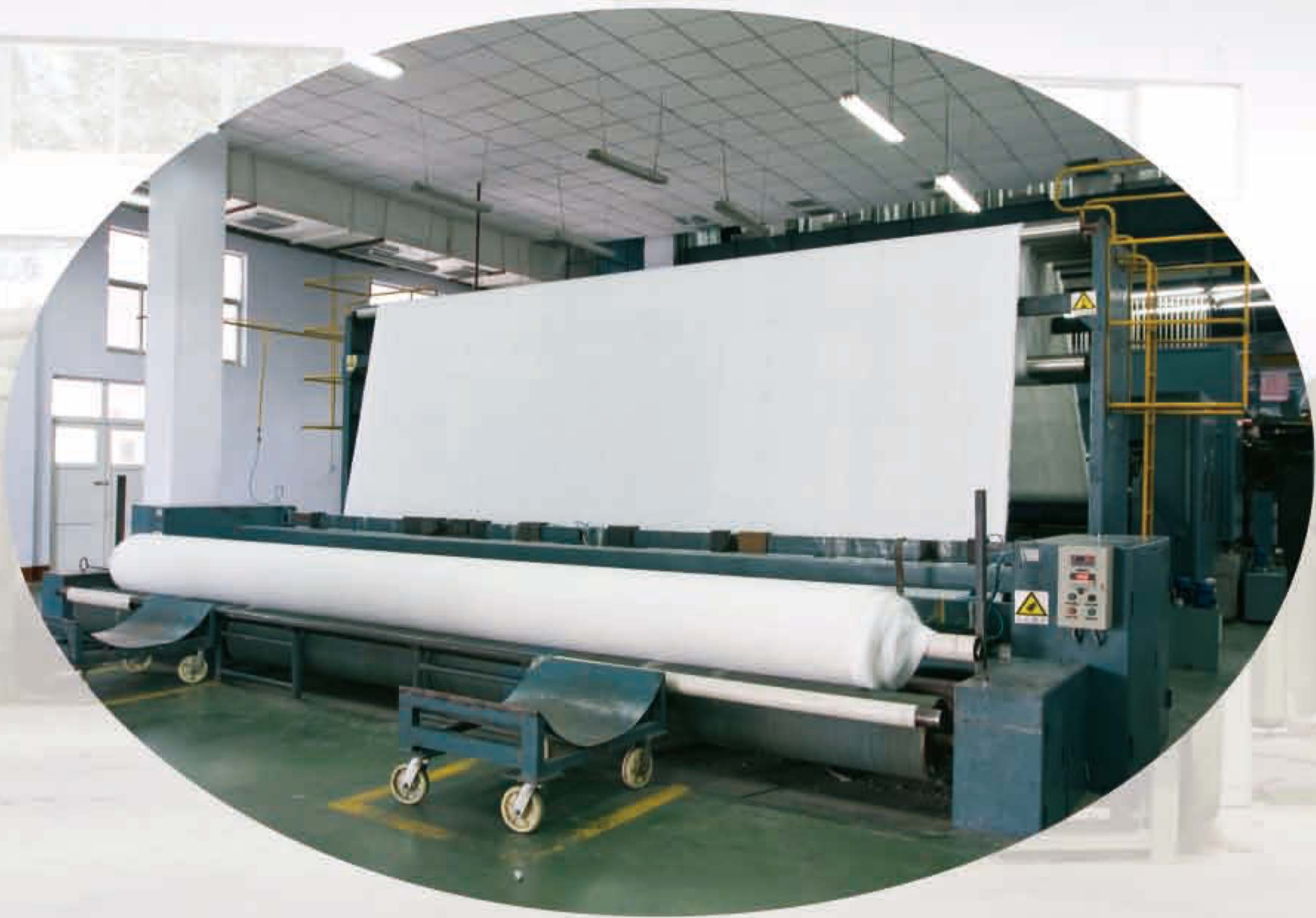
长丝纺粘针刺非织造土工布生产线 Falament spunbond needle punched geotextile production line.
